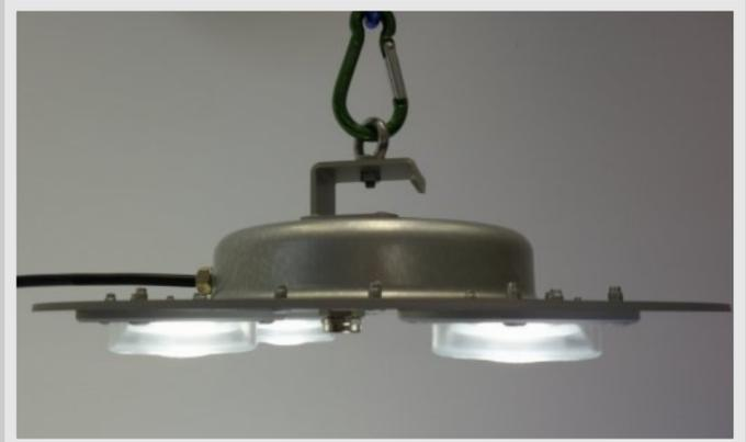
**Generation III** has fully vented housing. Therefore insensitive to sudden ambient pressure changes. Soft mounting of the electronics means high seismic capacity, no sensitivity to vibrations and excellent protection against water, hot steam and other chemicals.
