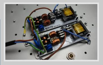
Proprietary electronics is based on full discrete design without integrated circuits, electrolytic capacitors and opto couplers. Predicted lifetime is more than 20 years. Mission profile 24/7 at 50 °C ambient temperature.
